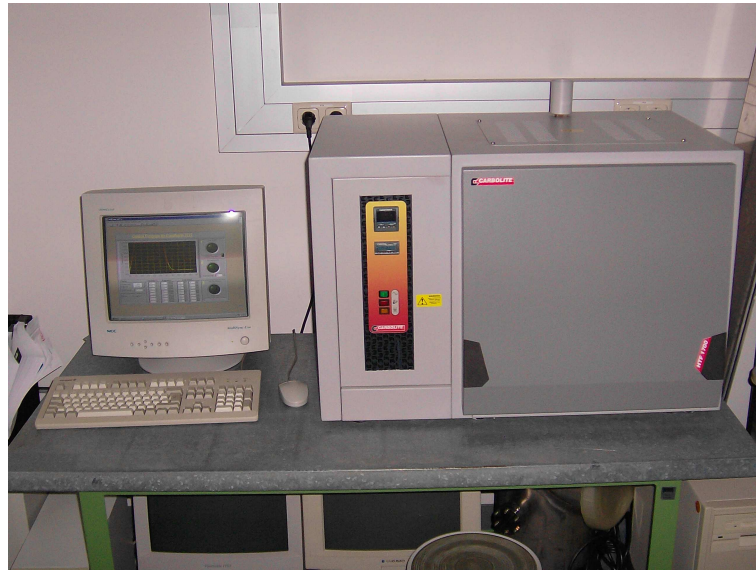
Figure 4.3: Photograph of the CARBOLITE™ HTF 1700 furnace which was used to perform the annealing of sapphire substrates.
