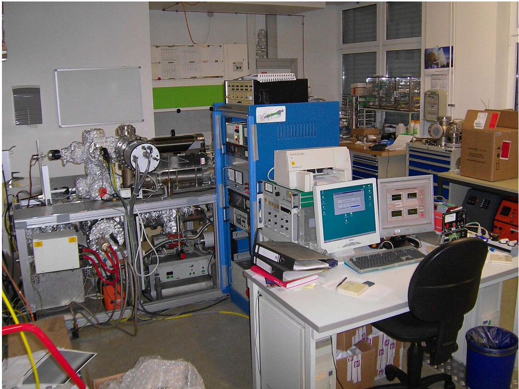
Figure 4.1: Overview of the sample preparation equipment constructed mainly from available vacuum components. Shown are the UHV electron beam evaporation chamber (at left), the HV argon ion beam milling chamber (at right; this also acts as an airlock system) and peripheral equipment. The computer screens on the table show the LabVIEW ™ computer control programs developed for the system.
