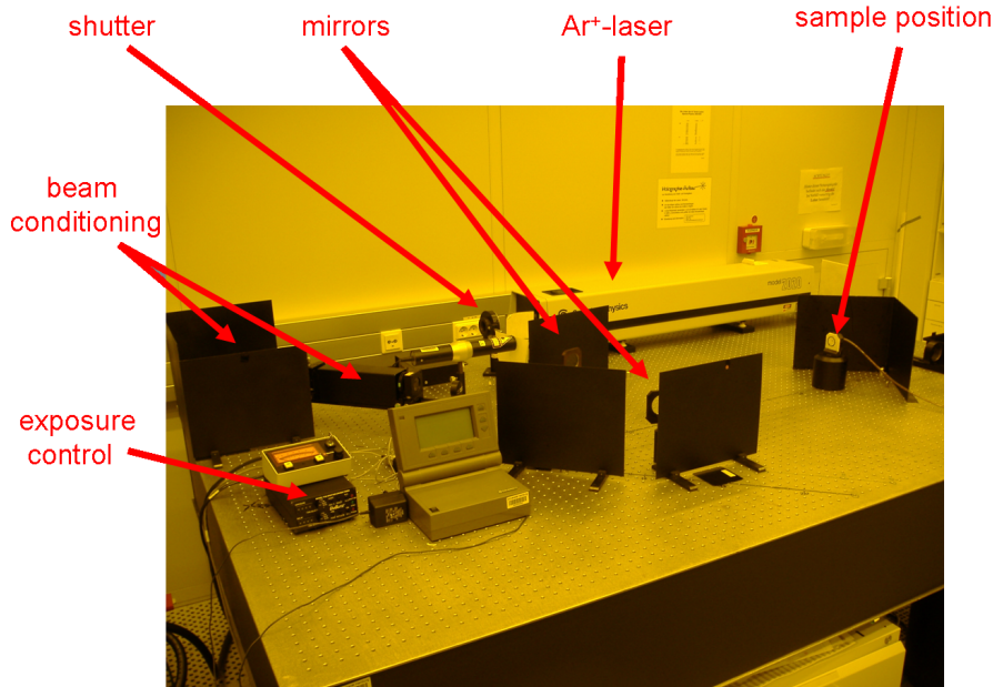
Figure 3.6: Labelled photograph of the laser interference lithography setup. The yellow tint is due to the light in the clean room. Visible are the Argon ion laser, the beam conditioning and exposure control setup and the deflection mirrors with the sample position (Photograph by Carsten Graf von Westarp). The beam splitter is located behind a black screen in the centre of the photo.
