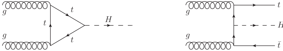
Figure 2.11: Production of a Higgs boson from gluons via a top quark loop (left) and an example for associated t\bar{t}H production (right).
