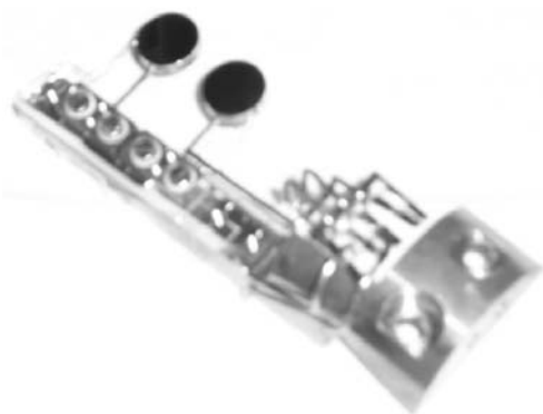
Figure 2.7: Photography of the sample holder: Assembly of Cu(100) and Cu(111) single crystals.
