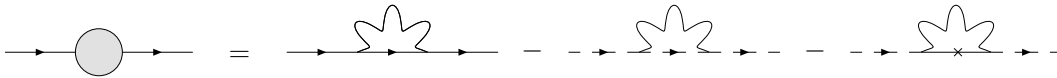
Figure 2.1: Renormalization of the 1-loop electron self-energy: From the unrenormalized loop correction, we subtract the same graph at on-shell external momentum (dashed) as well as the derivative with respect to the external momentum. This results in an insertion of a Dirac gamma matrix, indicated by \times .
