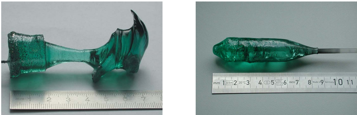
Figure 3.7.: Left: Prototype 15% Yb:YAG crystal #SK and right: Crystal #SNF, grown under optimised conditions using a seed crystal for defined orientation. Both crystals display a blueish turquoise colour due to the presence of colour centres formed by oxygen vacancies and \text{Yb}^{2+} , as is typical for as-grown crystals when grown under reducing conditions.
