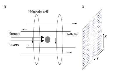
**Figure 10.2:** (a) Setup showing the propagation direction of the laser beams (large arrows) and the configuration of the magnetic trap. The Helmholtz coils generate the homogeneous Ioffe field oriented along the Z direction and the Ioffe bars the quadrupole field in the X - Y plane, shown in subfigure (b).
