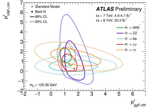
**Figure 2.7:** Likelihood contours measured for  $H \rightarrow \{\gamma\gamma, ZZ, WW, b\bar{b}, \tau\tau\}$  indicating the best-fit value to the data (+), 68% (full) and 95% (dashed) CL contours and the SM expectation. Fig. taken from Ref. [40]
