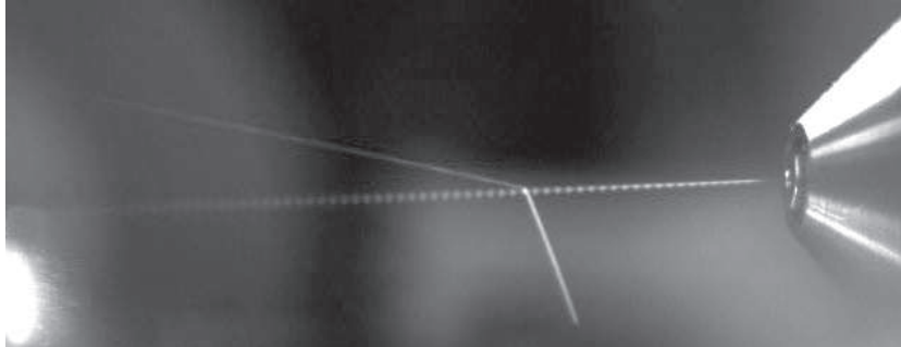
Figure 3.10: Modulated hydrogen jet ejected from the cryogenic nozzle into the vacuum chamber. One can see how a droplet collides with another droplet which has been reflected by the chamber walls and is substantially slower than the stroboscopic illumination. See also the appendix for a video of the source (figure A.3).
