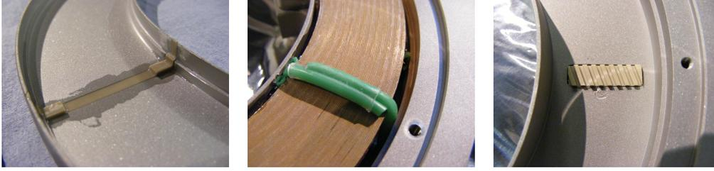
**Figure 4.11:** *Cooling channel design:* A 1mm high cooling channel is realised with peek and rubber spacers, leaving the cooling fluid in direct contact with the coil surface. On the left the slotted design of the moving coils is shown. In the middle the cooling channel is blocked with rubber tube between inlet and outlet. On the right a distance spacer for an unslotted cooling body design with slots for the cooling fluid can be seen.
