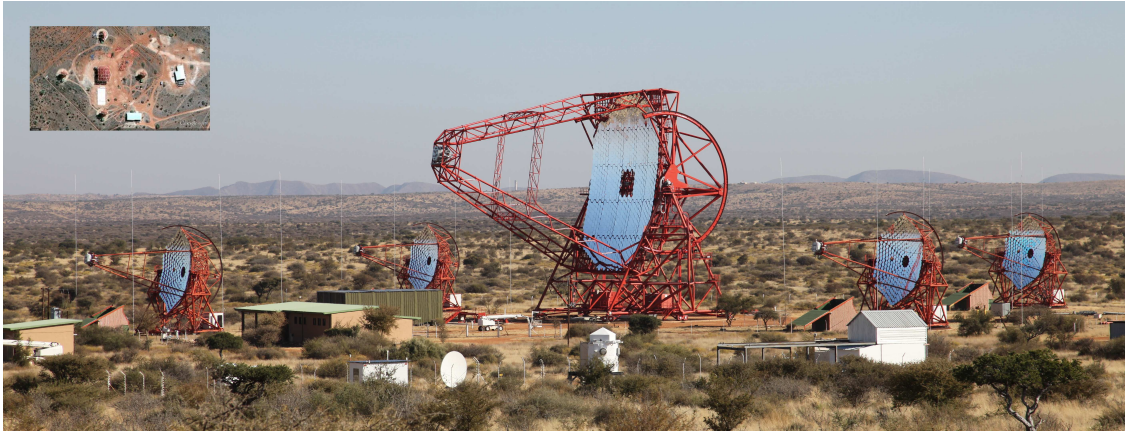
FIGURE 3.10 The High Energy Stereoscopic System (H.E.S.S.) in its phase 2 with the five Cherenkov telescopes (CTs). The four smaller CTs are named CT1 to CT4 and constitute the phase 1. The inlay shows a satellite picture from Google Earth of the H.E.S.S. array with its giant telescope CT5 in the centre of the quadratic layout.
