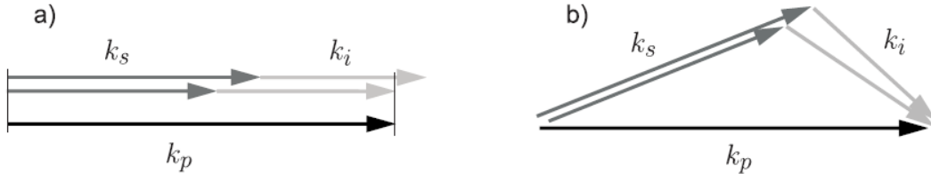
Figure 2.5: Schematic of a) collinear and b) non-collinear interactions of the pump and signal beam in the parametric amplification medium [45].
