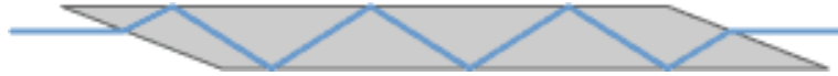
Figure 2.8: Zig-zag beam path in a slab crystal (side view) [30]. The seed beam is coupled into the crystal at brewster angled facets to keep the coupling losses low. The beam is then kept in the crystal by total internal reflection, following a zig-zag path in the laser crystal.
