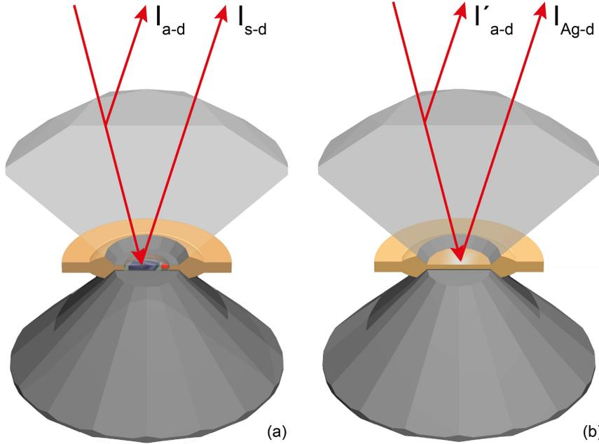
FIGURE A.6: **Absolute reflectivity retrieval in a DAC.** Panel (a) shows the reflected beams  $I_{a-d}$  from the air-diamond (*table*) and  $I_{s-d}$  from the sample-diamond (*culet*) interfaces in a typical DAC assembly. Panel (b) shows instead the  $I'_{a-d}$  reflected beam and the reflection  $I_{Ag-d}$  from an Ag non-drilled gasket used as a reference for our measurement.
