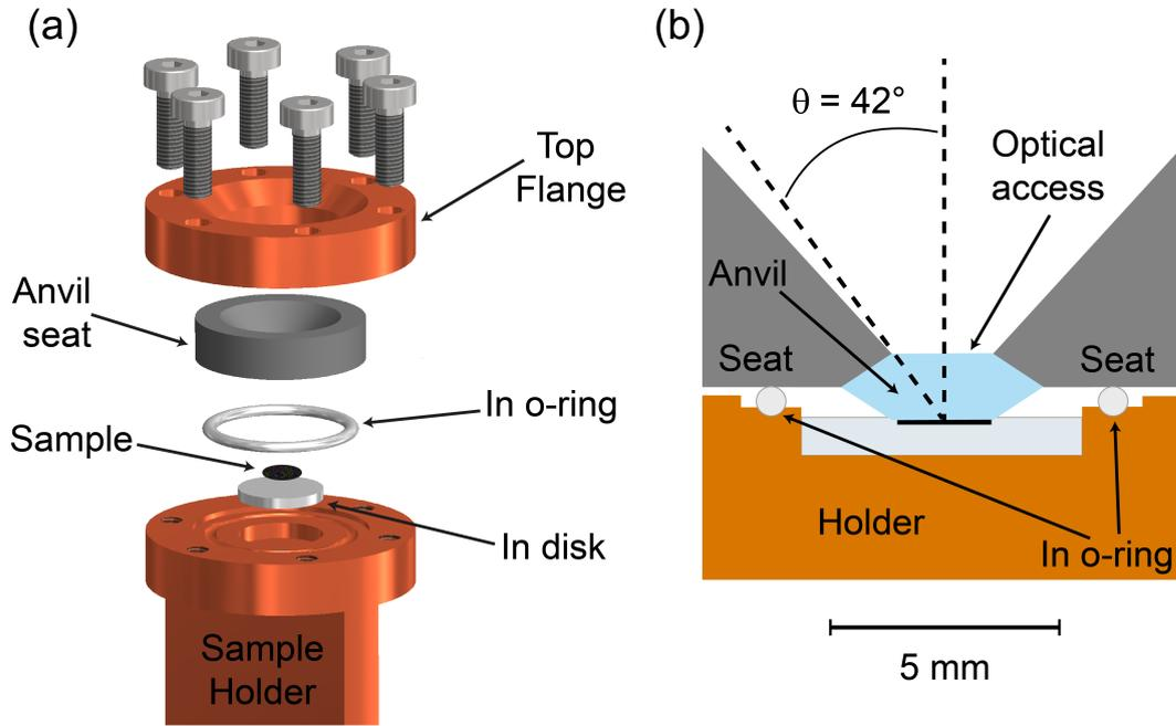
FIGURE A.16: **Sample holder for  $\text{K}_3\text{C}_{60}$  measurements.** Panel (a) shows an exploded view of the sample holder assembly conceived for the MIR pump-THz probe measurements. The lower part of the holder, connecting to the Oxford Optistat CF-V cold finger is not shown. Panel (b) shows a zoomed sketch of the sample holder assembly after closure. The black layer in contact with the anvil is the sample pellet, while the grey disk below is the In disk.
