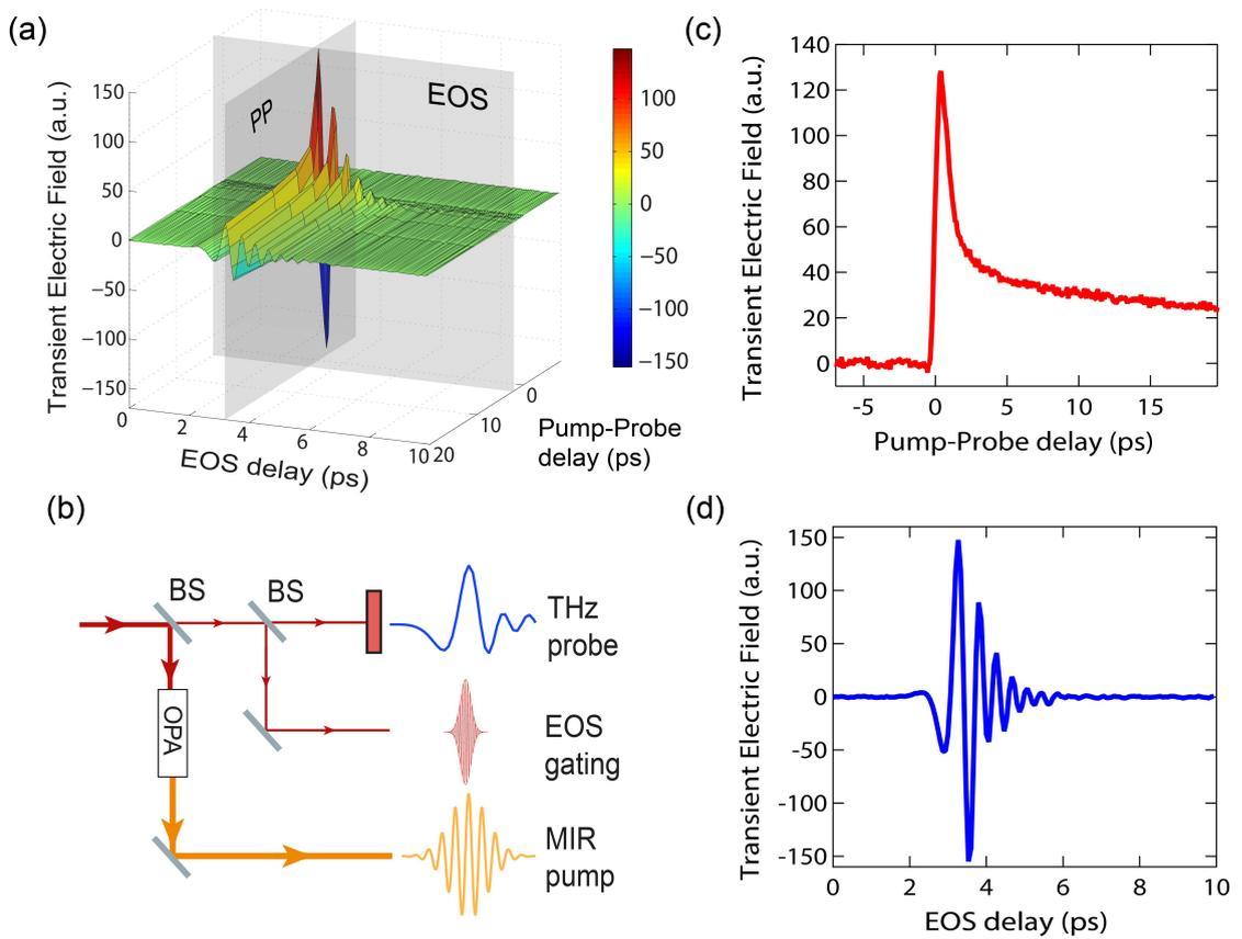
FIGURE A.11: **Example of THz time-resolved measurements.** Panel (a) shows the 2D time-resolved measurements of the MIR pump-induced changes in the electric field from a sample (in this case  $K_3C_{60}$  at 25 K). Panel (b) summarizes the arrangement of the beams involved in the measurement process. Panel (c)-(d) correspond instead to cuts of Panel (a) (respectively PP and EOS grey planes). All these data (averaged on 30 scans) are not normalized to the equilibrium reflected field.
