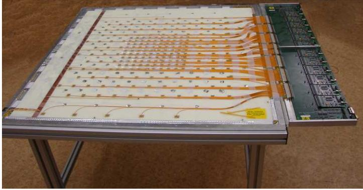
Figure 5.31: Picture of an opened AHCAL module with readout electronics.
