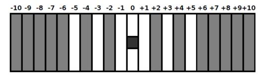
**Figure 6.8:** Default illumination pattern for images at the equator [217]. Stripes are numbered from left to right, starting with -10 and ending with +10. Grey stripes are switched off, white stripes are switched on. The dark square in the center indicates the opening for the camera.
