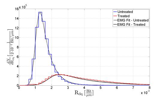
**Figure 8.12:** The x-axis shows the average boundary gradient  $R_{dq}$  measured with the algorithm and the y-axis shows the counts per bin.
