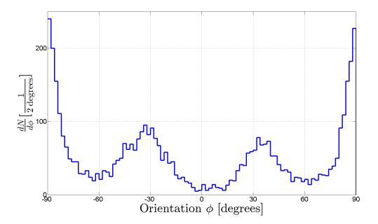
**Figure 8.11:** The x-axis shows the orientation of the boundaries in degrees. The y-axis shows the counts per 2 degree. The values used here are from the first equator of a treated cavity.
