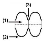
**Figure 3.3:** Schematic view of a two cell cavity. (1) is the cell, (2) depicts the equator and (3) the iris.
