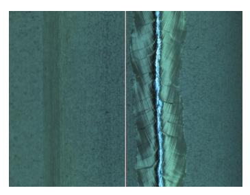
**Figure 8.3:** Image of the untreated cavity surface, equator 9. An offset between the image axis (white line) and the welding seam ridge of 1.8 mm is visible.
