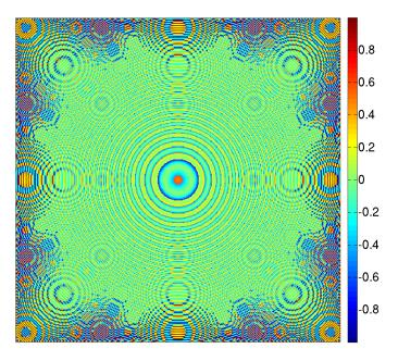
**Figure 7.12:** Difference image of Jaehne image and binary image. For each pixel, a difference between the intensity value of each pixel in the Jaehne image and the binary image is calculated and assigned to the pixel. The resulting image is color coded.
