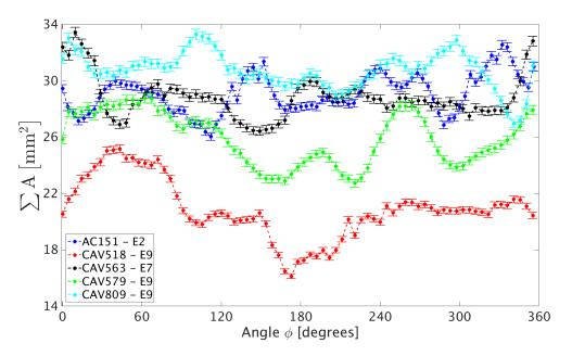
Figure 10.8: The total grain boundary area per image versus the image angle. The angular distribution of the optically worst equators of the five low performing cavities.
