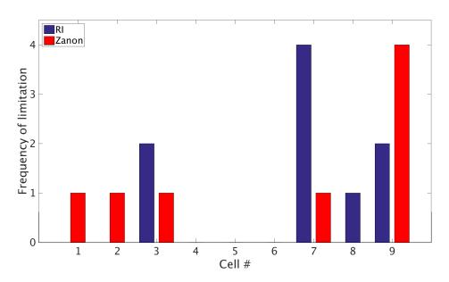
Figure 10.4: The longitudinal distribution of the maximum value of  $\sum A$  displayed for both vendors. The bars depict the measured occurrence.
