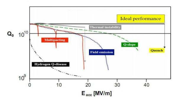
**Figure 3.6:** Schematic  $Q_0$  vs.  $E_{acc}$  plot. The x-axis shows the accelerating field in MV/m and the y-axis depicts the quality factor. The theoretical performance of a TESLA cavity should be a constant quality factor up to the thermodynamical limit of 55 MV/m. This theoretical behaviour is never seen, even in a defect free cavity [103].
