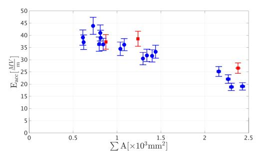
**Figure 10.7:** On the x-axis, the boundary area sum, which stands for a complete cavity, is shown, while the y-axis depicts the maximum accelerating field achieved by the respective cavity. The red squares display large grain cavities, the blue circles fine grain cavities.
