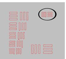
**Figure 7.9:** USAF1951 test chart after image processing. The red lines show the edges of the detected elements. The smallest separated group elements - encircled - are the elements of group five, elements one. This results in an resolution of 15.63  $\mu$ m.
