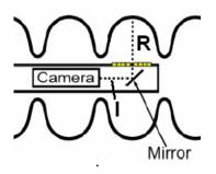
**Figure 6.6:** The focal length of the optical system f is the sum of the cell radius R and the camera-mirror distance I. The latter has to be adjusted to correct for deviations of the surface-mirror distance to keep the inner cavity surface in focus.
