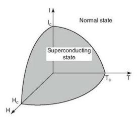
**Figure 3.1:** Three dimensional phase space of a superconductor. The material will stay in the superconducting phase if the current, the temperature and magnetic field are inside the volume of the shown phase space. An excess of one of the variables will lead to a breakdown of superconductivity [73].
