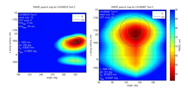
**Figure 10.5:** RMSE-Map of CAV518 (left) and CAV087 (right). The x-axis is the cell angle, the y-axis the longitudinal position along the cavity. The z-axis shows the color coded RMSE value. The most likely quench spot for CAV518 is about 44 mm below equator nine at  $(330 \pm 12)$  degrees and for CAV087 at equator nine at  $(141 \pm 16)$  degrees [213].
