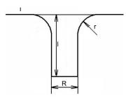
**Figure 3.11:** Geometrical parameters of a hole [133]. The bending radius r and the radius R are used to calculate the magnetic field enhancement.
