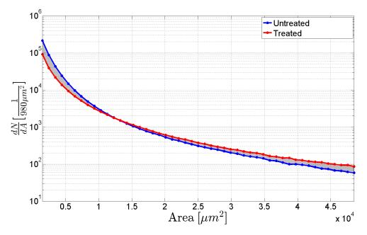
**Figure 8.6:** Grain boundary area distribution. The x-axis shows the boundary area, while the y-axis shows the count per  $980\mu m^2$ . The area distribution before (blue) and after (red) the surface treatment is shown.
