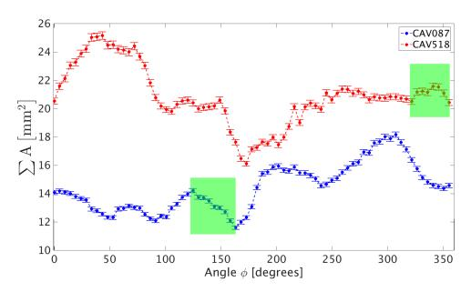
**Figure 10.6:** The total grain boundary area per image versus the image angle. The upper plot shows the distribution for CAV00518, the lower plot for CAV00087. The green boxes depict the most likely quench positions as obtained by second sound.
