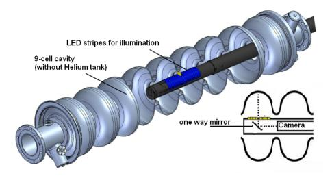
**Figure 6.3:** Drawing of the Kyoto Camera System used at DESY. The camera is viewing the inner surface via a 45° tilted half mirror. The distance to the mirror can be controlled for focusing. Behind this half mirror, three LEDs are mounted for the central illumination.  $2 \times 10$  acrylic strips with LEDs are mounted left and right from the opening in the rod for a more detailed illumination [216].
