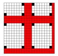
**Figure 7.21:** Test pattern with false positive pixels. The red pixels are true boundary pixels. Black pixels are false positive pixels of the boundary because of a higher intensity gradient than the average background pixels.
