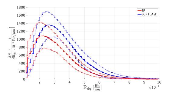
**Figure 9.7:** The x-axis shows the boundary gradient  $R_{dq}$  for boundaries within the welding seam region and the y-axis shows the counts per bin. The plots show the average  $R_{dq}$  distribution for all cells with a one  $\sigma$  interval. The red distribution is for RI and the blue distribution is for Ettore Zanon.
