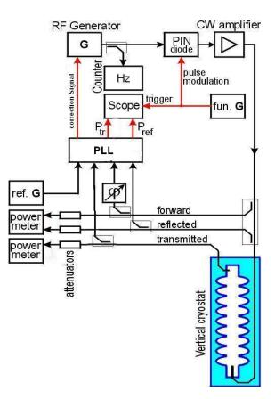
Figure 5.2: Schematic RF circuit of the vertical test stand at DESY [199].
