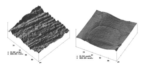
**Figure 8.1:** AFM images from niobium samples with a scanning area of  $100 \times 100 \ \mu m^2$  [255]. Left: Untreated surface sample. Right: Electropolished surface sample. A decrease in roughness but an enhancement of grain boundaries can be seen.
