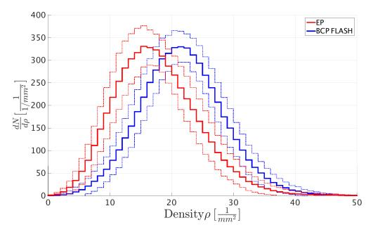
**Figure 9.2:** The x-axis shows the boundary density in the heat affected zone (HAZ), the y-axis the amounts of squares with a certain density. The plots show the average density distribution for all cells with a one  $\sigma$  interval.
