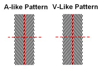
**Figure 8.9:** A schematic drawing of the two possible fishbone patterns. An A-like pattern will have boundaries left of the image axis with a positive angle w.r.t. the dotted line and the boundaries on the right will have a negative angle. The V-like pattern has mirrored characteristics.
