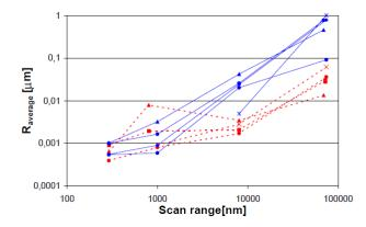
**Figure 4.5:** The average roughness as a function of the scan length, measured with an AFM. Cavities with EP are the red dotted lines, cavities treated with BCP are the blue full lines. The average roughness for small length scales (smaller than fine grain size) shows no difference while for larger length scales the roughness of EP cavities are about a magnitude smaller. [184].
