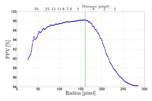
**Figure 7.15:** PPV as a function of the radius. On the lower x-axis the radius r is shown, while the y-axis shows the PPV for the corresponding circular region with radius r. The upper x-axis shows the distance between two consecutive boundaries at the corresponding radius. The green line depicts the best value and its corresponding radius.
