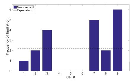
**Figure 10.3:** The longitudinal distribution of the maximum value of  $\sum A$ . The bars depict the measured frequency, the dashed line shows the expected frequency  $p_{0,c}$ .
