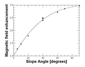
Figure 7.26: Magnetic field enhancement factor  $\beta$  versus the slope angle [132].
