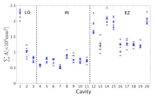
**Figure 10.2:** The total grain boundary area for each cavity in the dataset. LG stands for the three large grain cavities in the dataset. For each cavity, the values for all nine cells are shown.
