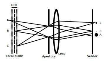
**Figure 6.4:** The points on the left side of the image (A,B,C) are projected onto the camera sensor by the lense and aperture. Depending on the position of the observed points, whether within our outside the finite DOF, they appear as bigger points on the camera sensor [217].
