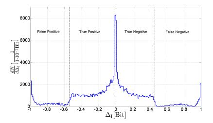
**Figure 7.13:** The plot shows the histogram of the pixel value distribution of the difference image. The corresponding classification intervals are depicted by dashed black lines.
