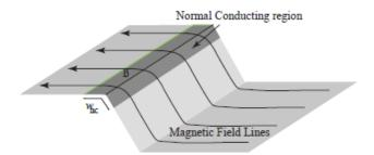
**Figure 3.10:** Schematic view of a quenched grain boundary due to magnetic field enhancement. The normal conducting region will decrease the quality factor, although the cavity itself will stay superconducting [132].
