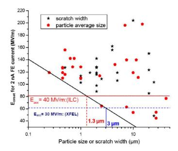
**Figure 3.8:** The onset electric field for 2 nA FE currents versus geometrical size of all identified emitters found on different fine grain, large grain and single crystal niobium samples [117]. The electric surface field is related to the accelerating field  $E_{acc}$  by a design depended constant, see table 4.1.
