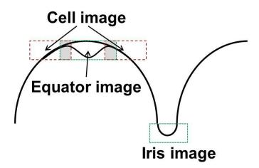
**Figure 6.2:** Image positions in a cavity. At the equators, the welding seam itself is in the central axis of the image - depicted by the green box. The cell images are taken with an offset of  $\pm$  8 mm relative to the equator position - depicted by the red boxes. The overlap region is shaded. The iris image is taken between the cells and at the beam pipe weldings. Sketch is not to scale.
