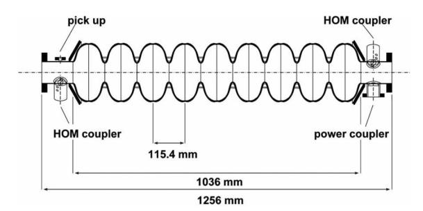
**Figure 4.1:** Schematic view of the nine cell cavity with main power coupler, pick up probe and two HOM couplers [34].
