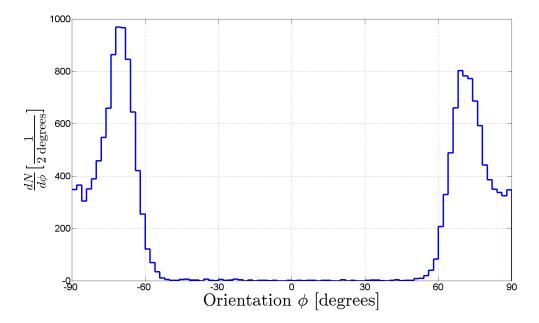
**Figure 8.8:** The x-axis shows the orientation of the boundaries in degrees. The y-axis shows the counts per 2 degree. The values used here are from the first equator of an untreated cavity.
