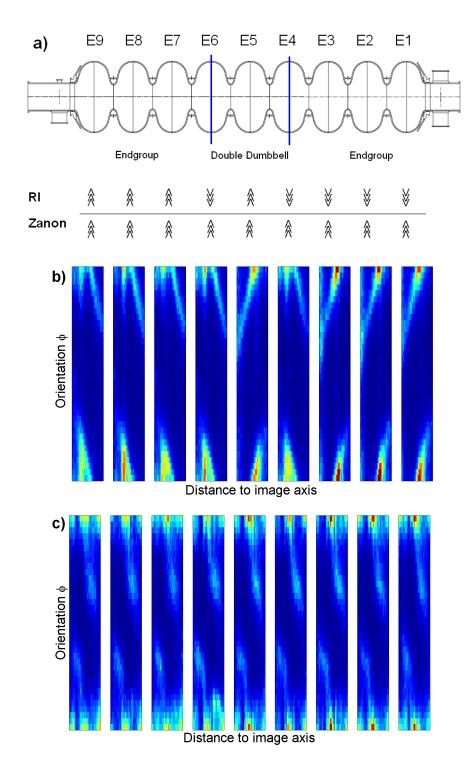
**Figure 9.6:** a) sketches the assembly procedure of a cavity at the two vendors and allows for the assignment of the patterns to the corresponding cells. Within the histograms, the color depicts the counts per bin. The x-axis shows the boundary centroid with respect to the image axis, only for the welding seam region. The y-axis shows the boundary orientation w.r.t. an axis perpendicular to the welding seam. b) is for RI and c) for Ettore Zanon.
