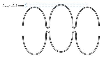
**Figure 6.7:** A cell symmetry axis can deviate from the geometrical axis up to 1.5 mm. The deviations are randomly angular distributed and each cell can be affected, leading to a individual camera position for each cell.
