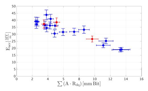
**Figure 10.9:** On the x-axis, the boundary area sum times the boundary roughness, which stands for a complete cavity, is shown, while the y-axis depicts the maximum accelerating field achieved by the respective cavity. The red squares display large grain cavities, the blue circles fine grain cavities.
