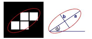
**Figure 7.16:** On the left side, a four pixel object and the ellipse with the same second central moment is shown. On the right side, the ellipse with its major axis a and minor axis b and the horizontal z-axis for the angle assignment is shown.
