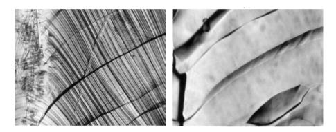
**Figure 8.2:** Optical microscope image of the same welding seam surface  $(1770 \times 1370 \ \mu m^2)$  [176]. Left: Untreated cavity. Right: BCP treated surface. The fishbone pattern (left image) are thin lines going from top left to bottom right. The grain boundaries are also visible but not dominant. The grain boundaries (right image), going from bottom left to top right, show a preferred orientation.
