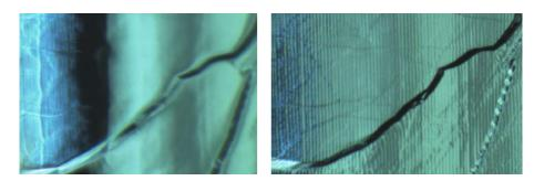
**Figure 7.22:** OBACHT image of the same boundary after EP (left) and BCP (right) [217].
