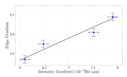
**Figure 7.23:** The x-axis shows the intensity gradient of a boundary derived from the image and the y-axis the geometrical gradient measured with the profilometer. The linear fit with the equation is shown.
