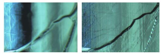
**Figure 9.1:** OBACHT image of the same boundary after EP (left) and BCP (right) [217, 254]. The observable boundary area changed due to the treatment.
