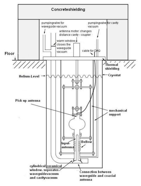
**Figure 5.1:** Schematic view of the vertical test stand at DESY [96]. For a better overview, only a single cell cavity is shown.
