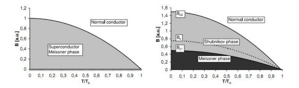
**Figure 3.2:** The phase space diagrams for type I (left) and type II (right) superconductor are shown. The x-axes show the normalized temperature while the y-axes depict the external magnetic field in arbitrary units. For type I superconductors, an increase above  $B_C$  will induce the normal conducting phase. For type II superconductors, magnetic vortices can penetrate the material above  $B_{C,1}$  and a mixture phase of superconductivity and magnetism occurs.
