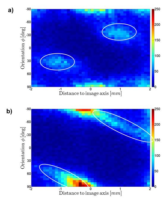
**Figure 9.5:** The x-axis shows the boundary centroid position with respect to the image axis. The y-axis shows the boundary orientation  $\phi$  in degrees w.r.t. an axis perpendicular to the welding seam. Only the welding seam region is shown. The upper plot (a) represents boundaries in the welding seam region of a Ettore Zanon cavity, the lower plot (b) of a RI cavity. The white ellipses encircles the welding seam boundaries. The color depicts the counts per bin.
