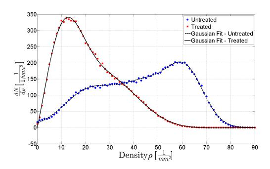
**Figure 8.4:** Grain Boundary density distribution. The x-axis shows the boundary density. The y-axis shows the amount of squares found with the respective density per equator. The blue dots describes the distribution before, the red squares after surface treatment. The distributions are sums of two Gaussian distributions, which are depicted by black lines. See figure 8.5 for the spatial distribution.
