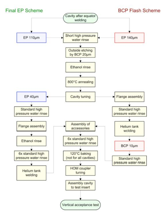
**Figure 4.3:** Process flow of surface treatment for cavities including helium vessel welding. The two different flows are for EP and for BCP preparation cycles. [154].
