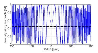
**Figure 7.11:** Line profile across the Jaehne test image g. The threshold of 0.46 Bit is represented by the black dashed line. Each boundary pixel above this line is considered as a boundary pixel. Note the center disk at r<16, which is defined as boundary pixel, although it is a diffuse background region. This will lead to false positives for small r and drop the accuracy within this region.
