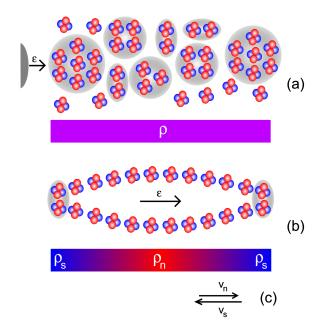
**Figure 5.5:** Energy propagation in superfluid helium. In (a) the density equilibrium of the two fluid-components is distorted by the deploying of an amount of energy  $\varepsilon$  into the superfluid. The energy leads to a break up of superfluid components and a local rise of the normal fluid. Therefore a superfluid counterflow takes place, and the two flows cancel out each other concerning a net mass flow but the entropy will spatially oscillate [201].
