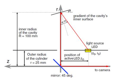
**Figure 6.9:** Schematic view of the illumination model [215]. With given properties of the cavity and acquisition geometry, the incident angle  $\theta$  of the grain boundary can be calculated.
