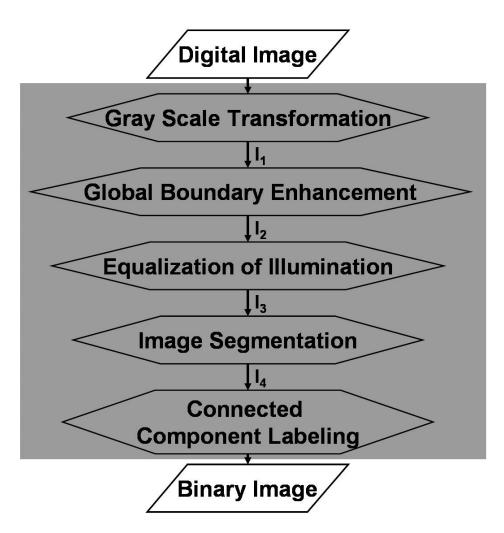
**Figure 7.1:** Flowchart of the developed algorithm for image processing. The output of the algorithm is a binary image. The image processing algorithm is depicted by the gray rectangle. The indices  $I_i$  refer to intermediate pictures. Both, the binary image and the original digital image is used for further image analysis.
