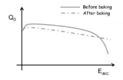
**Figure 4.6:** This schematic sketch shows two Q vs E curves of the same cavity. One depicts the curve progression before and one after baking [168]. A sudden increase of losses at high fields is visible, which is then removed after baking.
