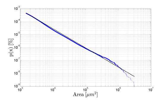
**Figure 8.7:** This double logarithmic plot shows the probability of occurrence of a grain boundary area versus the very grain boundary area. The blue squares depict the experimental found distribution, the black dashed line the power law fit.
