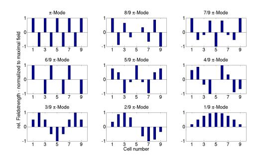
**Figure 3.5:** Electric field amplitudes for the passband eigenmodes of a 9-cell TESLA cavity.
