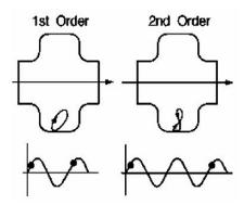
**Figure 3.7:** One point multipacting in a cavity of first and second order where the n-th order describes the numbers of RF periods between the impacts. Two point multipacting is the resonant travel of electrons between to distinct regions (not shown) [75].
