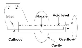
**Figure 4.4:** Schematic for horizontal EP. A membrane pump drives the acid mixture through a cooling and filtering system. From there it reaches the inlet in the aluminum cathode and fills the inside of the cavity. The acid flows back into the system via an overflow. At the end of the treatment, the cavity must be tilted to remove the complete acid. [189].
