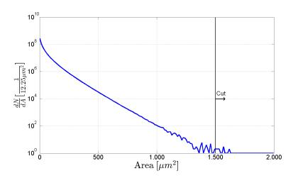
**Figure 7.5:** Pixel noise distribution. On the x-axis the area of the objects found in the binary images is shown. On the y-axis the counts per bin are displayed on logarithmic scale. This histogram contains the sum of 1000 images. Objects below an area of 1500  $\mu$ m<sup>2</sup> are cut.
