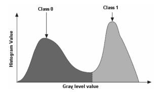
**Figure 7.4:** Gray scale histogram. Two classes of pixels can be identified in the histogram [243]. Class 0 are background pixels and class 1 are foreground pixels. The optimal threshold to separate these classes can be found by calculating the intra-class variances as a function of the threshold. The optimal threshold is the one which minimizes these variances.
