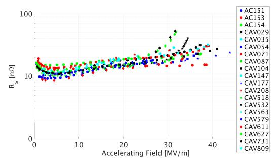
Figure 10.1:  $R_s$  versus  $E_{acc,max}$  diagram of the used dataset. The applied accelerating field is shown on the x-axis, the y-axis shows the corresponding surface resistance measured in a cold RF test.
