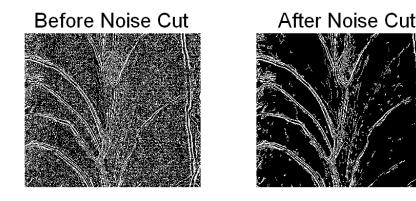
**Figure 7.6:** The left image shows an image section of the binary representation before the area cut to remove the noise, the right image the same image section after objects with an area smaller than 1500  $\mu m^2$  are removed. More than 99.8 % of objects in the image was removed.
