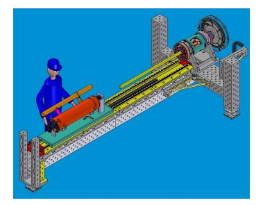
**Figure 6.1:** 3D sketch of the OBACHT set up. A cavity with helium tank (orange) is mounted on the movable sled (turquoise), which is located at the mounting position. The camera rod (yellow) can be rotated with the torque motor (turqoise/gray).
