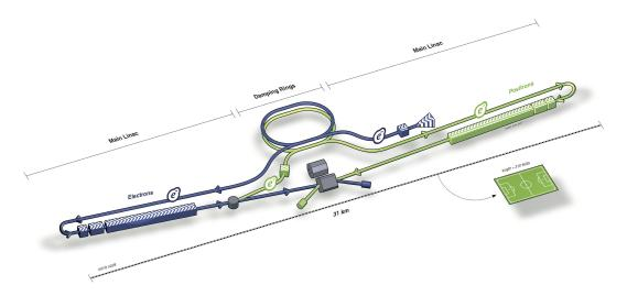
**Figure 2.3:** Schematic view of the ILC The linear accelerator will have a length of  $2 \times 8$  km [16].
