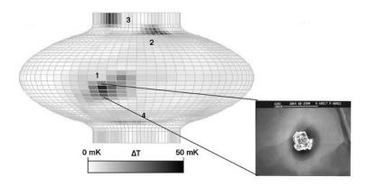
**Figure 5.4:** Temperature map of a 1.5 GHz single cell cavity. The heating at the quench site (1) and field emissions at (2-4) is shown. A SEM picture of the RF surface taken at the quench site is shown at the right [205].
