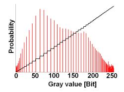
**Figure 7.3:** Contrast enhanced histogram (original figure 7.2). The CDF is linearized via adaptive binning of the PDF.
