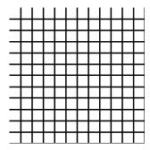
Figure 7.19: Test pattern with squares of a side length of 22 pixels and 3 pixels thick boundaries and a total area of  $300 \times 300$  pixels.
