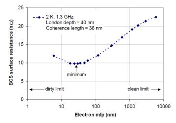
**Figure 4.2:** BCS resistance as a function of the mean free path. A minimum is observed at  $\ell \approx \xi$  which equals and RRR of 10. [105]
