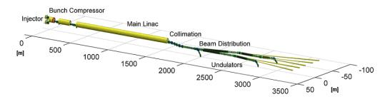
**Figure 2.2:** Layout of the XFEL. The acceleration section will have a length of 1.2 km. A beam delivery system will distribute the accelerated electron beam into five distinct tunnels with undulators to generate intense laser pulses [34].
