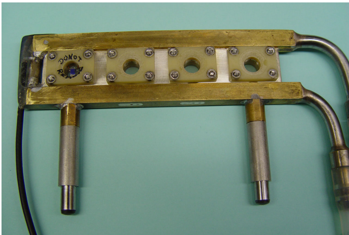
Figure 2.6: Image of a sample holder with three sample cells. The leftmost cell contains a temperature sensor. The tubing on the right can be connected to a water bath.
