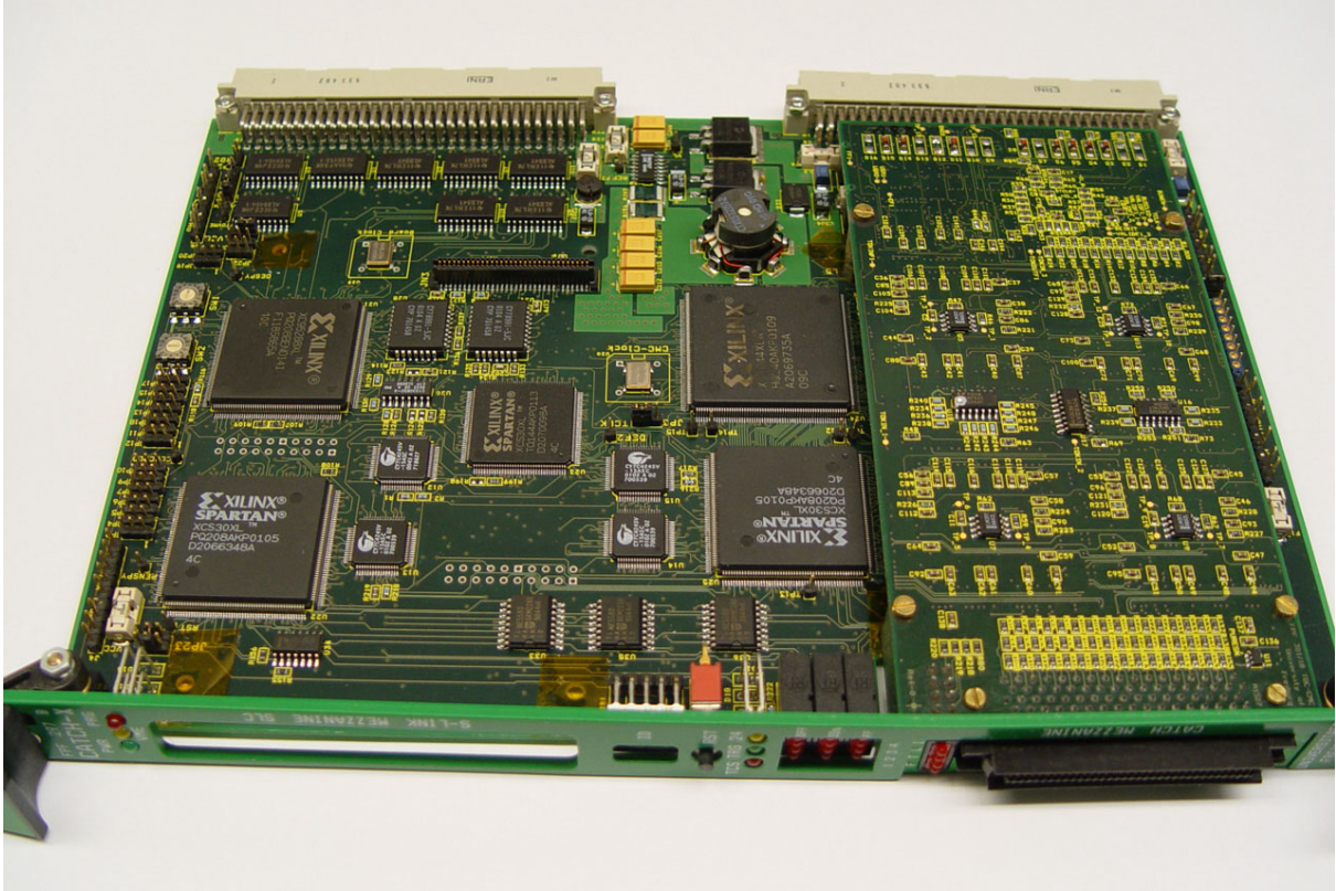
Figure 4.15: The 6U-VME TS-TDC based on the Catch-X with a F1-TDC mezzanine card (right slot).
