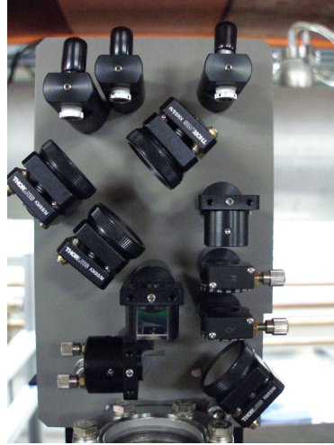
Figure 4.11: Picture of the optic components mounted on the base plate of the electro-optic frontend. The vacuum window can be seen on the bottom as the whole frontend is installed above the electron beam pipe.
