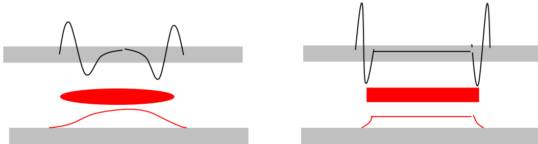
Figure 6.2.1 Coupling of the beam to the pickup for an elliptical beam (left) and for a flat beam (right) is shown on the top in black. The charge distribution of the beams is shown on the bottom in red. The beam is directly under the pickup.
