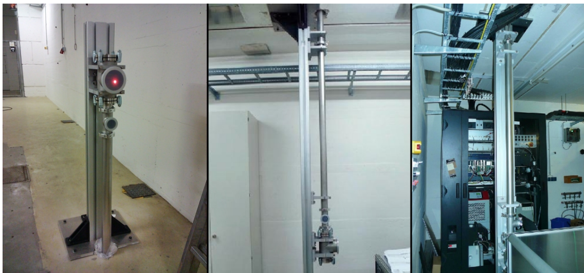
Figure 15: Laser beam transfer systems, which guide the optical beams to the accelerator. Left: upper part of the pump-beam-transfer. This image shows when the laser beam was transmitted to the upper floor for the very first time. Middle: lower part of the pump-beam-transfer. Right: Lower part of the probe-beam-transfer.
