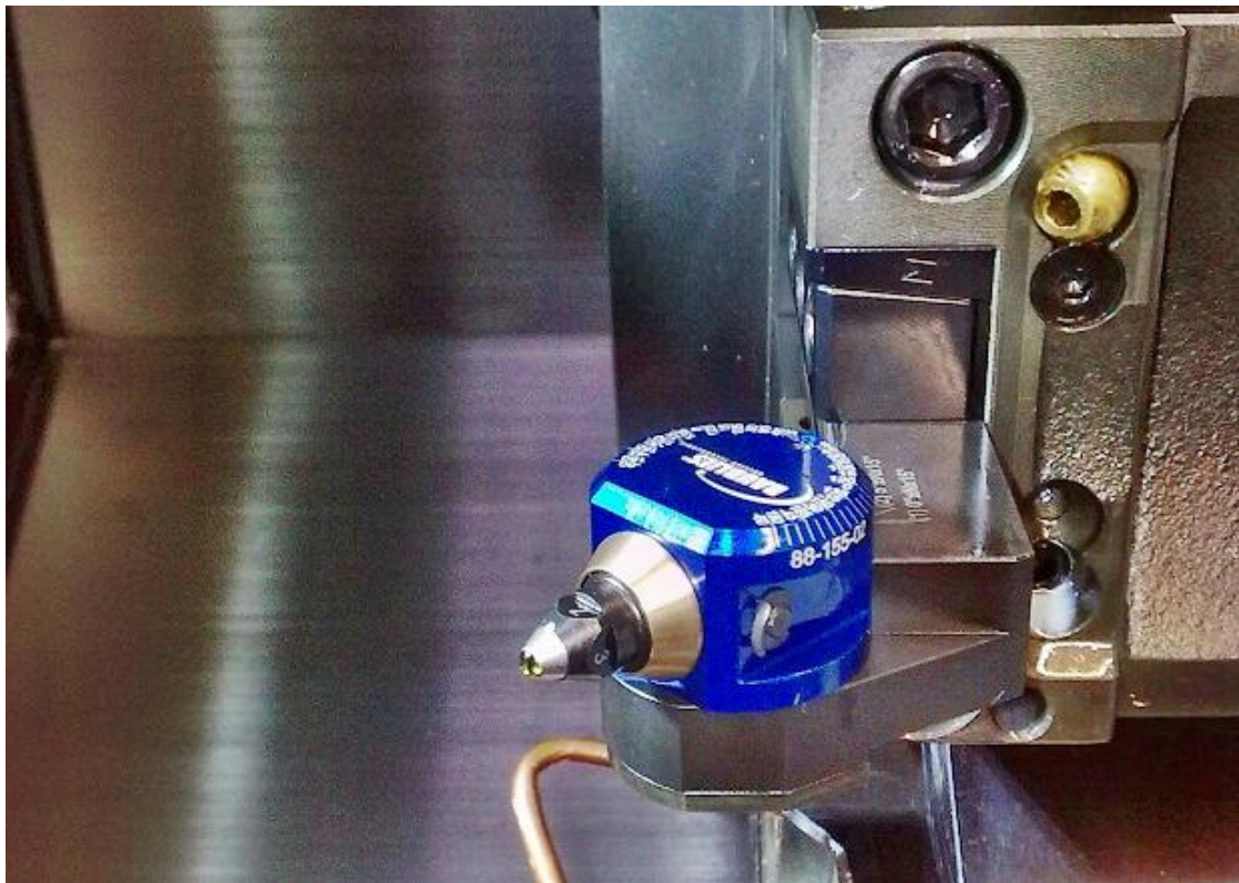
Figure 40: Artificial diamond on a flexible holder, which was used to flatten the surfaces of the high voltage electrode parts. The tool was purchased from the Baublies AG [Baublies-AG (2007)]. The pictures shows the actual usage in one CNC machine on DESY ground.
