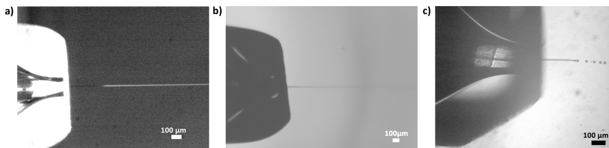
Figure 5.7: Three microscope images. a) 1st microscope in in-line geometry. b) 2nd microscope under 45°. c) 3rd microscope employing stroboscopic light and high magnification.
