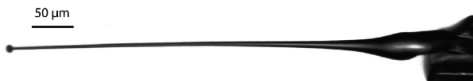
Figure 3.4: Microscope image of a supersonic microjet with v_{\text{jet}} = 490 \frac{\text{m}}{\text{s}} . The edge of the capillary is at the right side and the jet is visible at the left side. The laser illuminates the liquid in the capillary. It is not visible in this figure. Image is adapted from: Tagawa, Y. et al. Phys. Rev. X 2, (2012), 031002.
