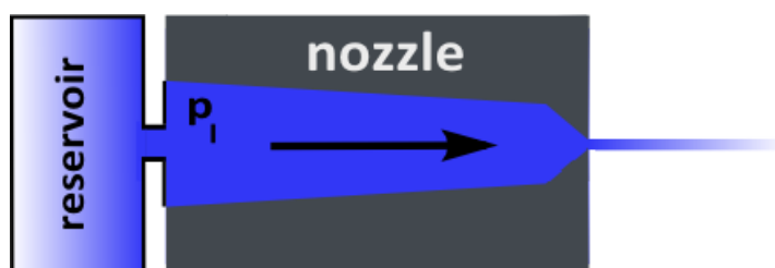
Figure 3.2: Scheme of a Rayleigh nozzle.
