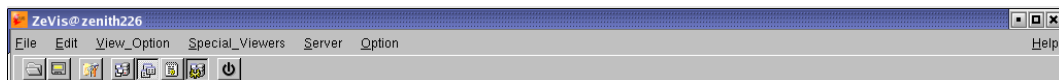
Figure 5.14: A new Iconbar, which presents the necessary functionality from the old Toolbar and some actions from the main Menubar "File" section such as "Open" root file, "Save" an event display image, "Exit" the program, and from the "View_Option", "EasyTool".
