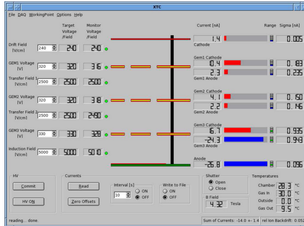
Figure 8.9 A screen shot of the user interface of the xtc software. The field values are shown on the left, while the output currents on each surface can be read from the right panel. Figure is taken from Ref. [195].
