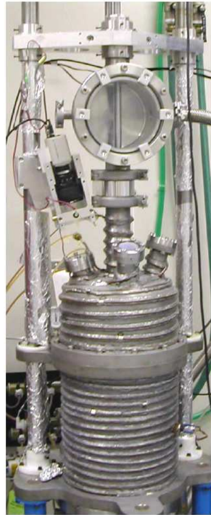
Figure 3.3: Chamber for Czochralski crystal growth at the University of Pisa. The distinction between the upper area, equipped with a large window, separated by a valve from the lower main chamber is shown.
