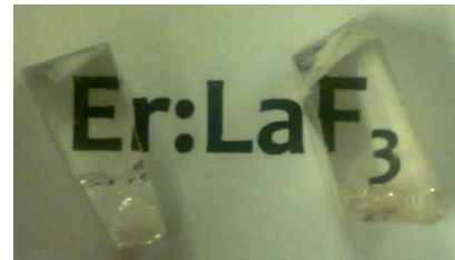
Figure 4.5: 0.6% \text{Er}:\text{LaF}_3 sample belonging to L (see Tab. A.3).
