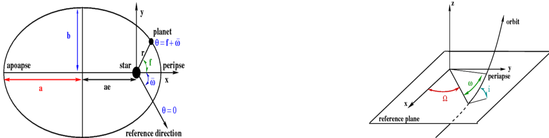
(a) A ellipse based on the radius of Eq. (2.1). The value of a stands for the semi-major and b the semi-minor axis. The eccentricity is e and the longitude of periastron passage is \bar{\omega} . The argument of periastron is \omega and f is called the true anomaly
