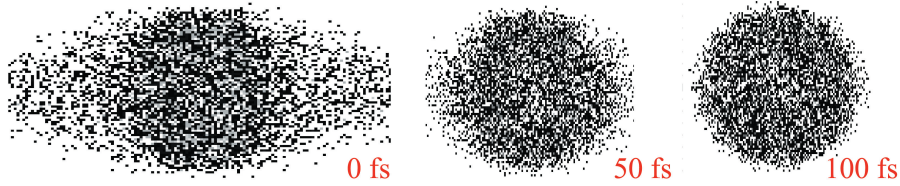
Figure 6.6: Simulated electron beam images on the detector after interaction with a 60 fs laser pulse. The electron beam is stripped by a 30 \mu\text{m} pinhole before interacting with the laser beam (25 \mu\text{m} beam diameter, 60fs, 1 mJ/pulse). The image shows the scattering with different time delay (0 fs, 50 fs and 100 fs). ASTRA simulation based on REGAE, see Appendix A.
