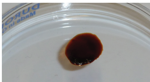
Figure A.15: Oil-like film left upon thawing of a single crystal of L-serine, irradiated for 14400 seconds.
