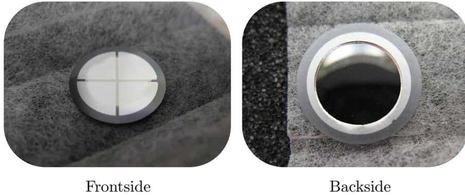
Figure 6.15.: Photographs of the X-ray Beam Position Monitor (XBPM). **Left:** Frontside, **Right:** Backside. [By Courtesy of B. Steffen].
