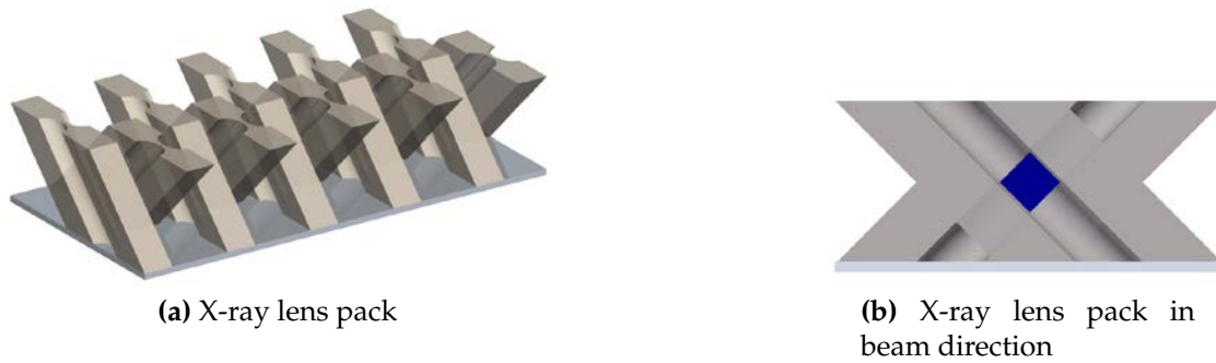
Figure 2.10: Crossed X-ray lens layout of a CRL (a) and in cross sectional view (b). The one dimensional focussing segments alternate in orientation by 90^\circ in order to create a two dimensional focus [117] (illustration from [104]).
