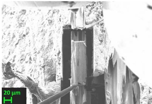
(a) Attached to the manipulator (FIB image (30 kV, 50 pA), 5 mm WD, SE2-detector)
