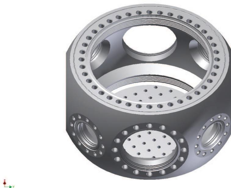
Figure 3.1.: CAD model of the vacuum chamber used to build the "Test chamber"
